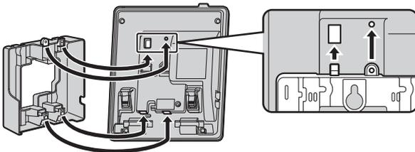
2. Fasten the wall mounting adaptor to the base with the small screw.
